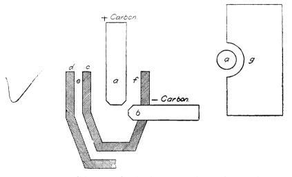
two crucibles, was filled with magnesia. g is one of two carbon plates, 1.5 cm. in thickness, which served as a cover.
